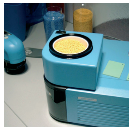
Fig. 5. Equipment for measuring plastics granules (photo: Byk-Gardner)
