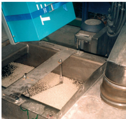
Fig. 9. Colour checking and classification of compounded plastics (photo: X-Rite)
