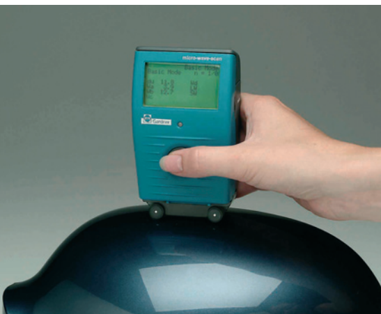
Fig. 4. New measuring principle rules out any influence exerted by the direction of measurement (photo: Byk-Gardner)
