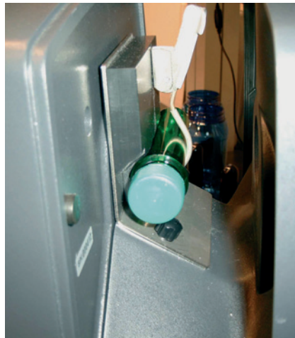
Fig. 7. Detail of colour measurement of a plastic preform (photo: X-Rite)
