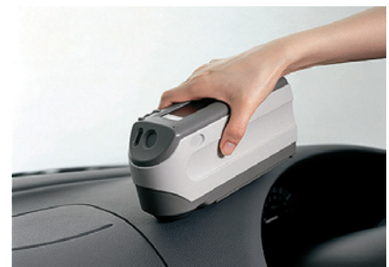
Fig. 2. Colorimeter with 45°/0° measuring geometry (photo: Minolta)
